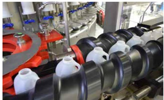
All rotary fillers can be combined with a pre-heating, bottle rinsing or decontamination unit and a capper/sealer to form a monoblock machine. This configuration reduces the footprint and change-over time, resulting in higher efficiency.
